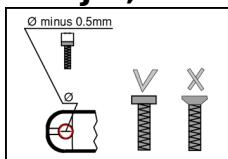
1. EN Warning: During installation, use appropriate screws / bolts. Make sure their head diameter is at least 0.5mm smaller than the hole diameter in the lamp. Use screws and bolts with a flat head base.
