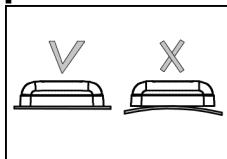
1. EN Always mount the lamps on flat surfaces if the set does not include a washer with the appropriate profile.
