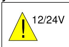
1. EN Warning: The lamp is designed for use only in installations with a DC voltage range of 12V - 24V.
