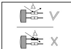
1. EN Warning: Secure the lamp connection to the vehicle installation carefully. Water ingress into this connection may cause damage to the lamp or the vehicle installation. Do not cut the tinned wire ends.
