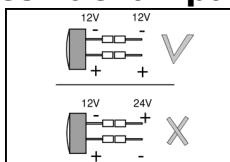
1. EN Warning: Pay attention to the correct connection of the lamp to the installation. Check the voltage compatibility in the installation with the voltage the lamp can operate with. Be careful not to reverse the power supply polarity.
